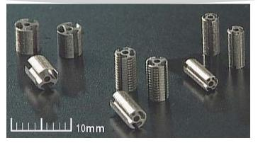
LASER FASTEC TECHNOLOGY is the one which is developed for mass-production of high-precision small sized motor core by YAG laser in stacking lamination. The regulation of product shape has a tendency not to be influenced and the small sized lamination core which can not be made so far can be mass -produced with stable strength and quality.
