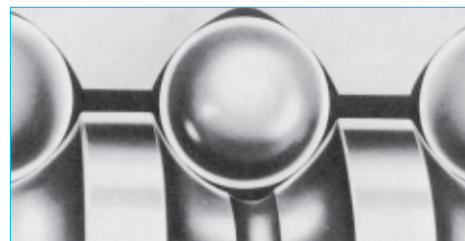
Figure 2: Ball screw groove profile
