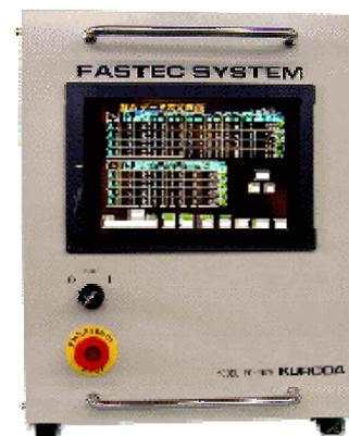
The FASTEC system consists of the dies for stamping core laminations and the control box for setting following functions.
