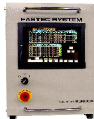
The FASTEC system consists of the dies for stamping core laminations and the control box for setting following functions.
