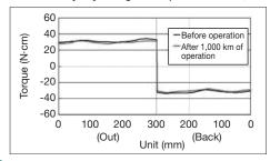
Delivers stable torque characteristics even during oscillating operation.
