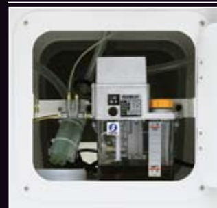
室温に同調した新しい潤滑油を摺動面へ供給する独立常温集中潤滑ポンプ Normal temperature new oil is constantly supplied. Sole collective lubricate oil device for each slides.
