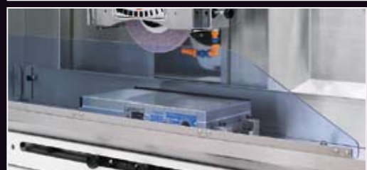
視認性がよく、安全に作業・確認ができる透明カバー Easy-to view and safety machining can be available by a transparent cover.
